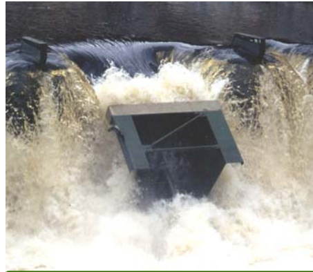
THIS IS A LIFE-SIZE MODEL SHOWING FUSEGATE TIPPING DURING ARTIFICIAL FLOOD TEST CONDUCTED AT ST. HERBOT DAM IN BRITTANY.
