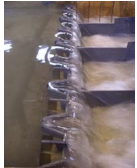
Small (above) and large (right) hydraulic models for Jindabyne Dam.
